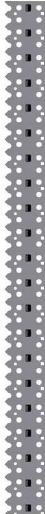
Template for punching and keeping the correct pitch
